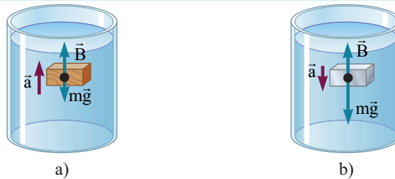
Figure 29. a) A totally submerged object that is less dense than the fluid in which it is submerged is acted upon by a net upward force. b) A totally submerged object that is denser than the fluid sinks.
