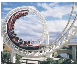
Figure 28. Passengers on 'corkscrew' roller coaster experience a radial force toward the center of the circular track and a tangential force due to gravity
