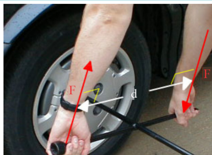
Figure 21. A mechanic applies equal and opposite forces at the opposite end of a 4-way wrench.
